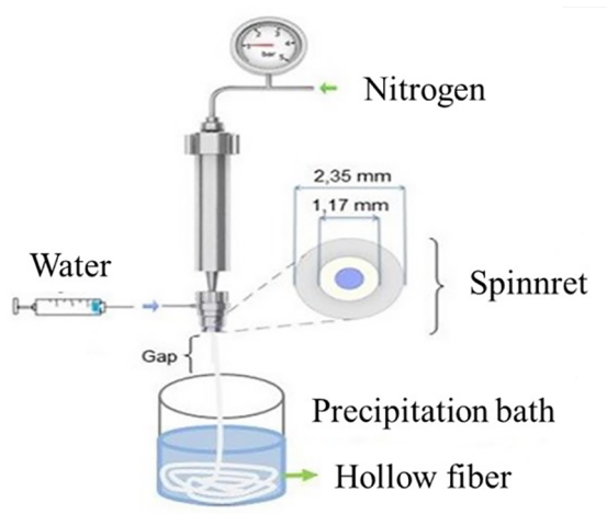
Figure 1. Schematic representation of the extruder and the hollow fiber membranes process 18 .
