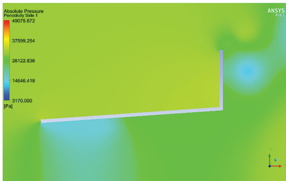
Figure 11: Pressure (a) and velocity magnitude (b) fields on the flanged diffuser for a H = 3.0 m depth.
