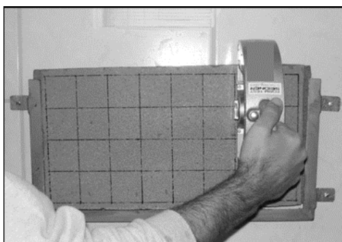
Figure 4 - Conduction of the Pendulum Rebound Hammer test
