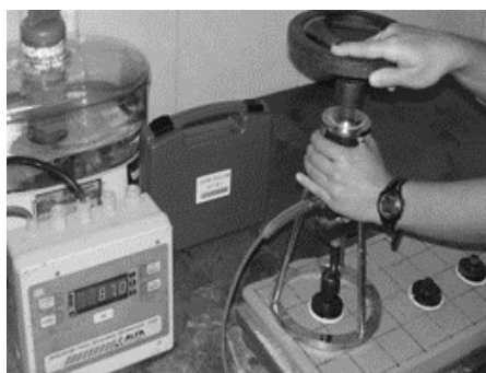
Figure 3 - Conduction of the superficial tensile strength test
