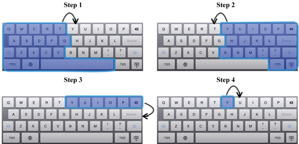
Figure 5. Three-dimensional scanning method in 4 steps. This method highlights blocks of keys. Once the user selects a block system performs line and column scanning method.
