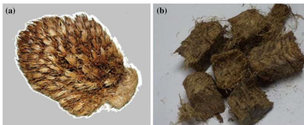
FIGURE 10. Empty bunch (a) and respective fragmentation (b) used in gasifier for energy production. Source: Ariffin et al. (2016)
