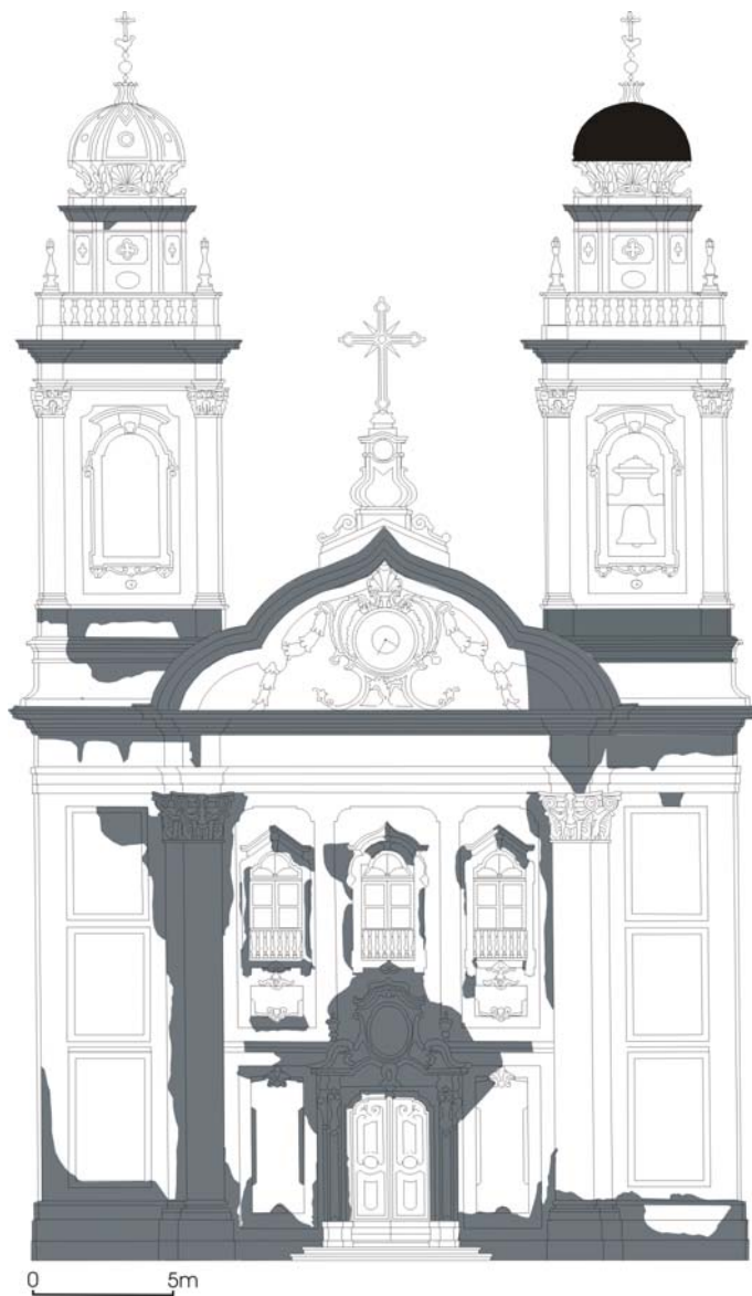
Fig. 2 – Distribution of black crust on the church of Ordem Terceira de Nossa Senhora do Monte do Carmo façade.
