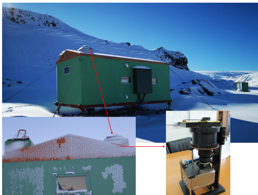
Figure 2. Punta Plaza module with two domes, and the FotAntar-4 (similar to the FotAntar-3) on the bottom-right side.
