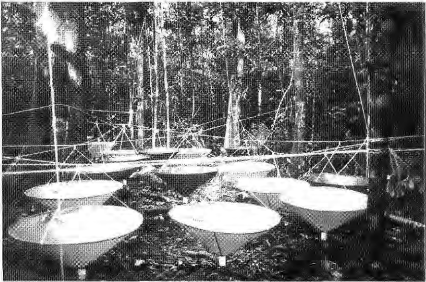
Figure 2. Funnel-shaped collecting trays are suspended from ropes under the canopy of Goupia glabra (Cupiuba 59; photo J. Adis)
