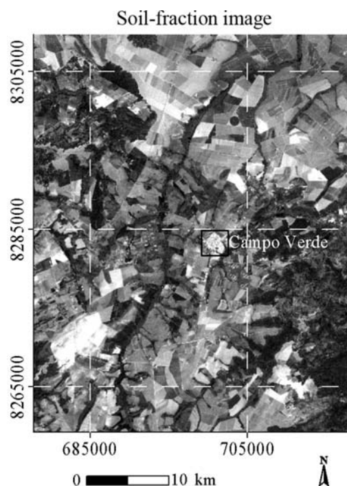
Figure 1. Soil-fraction image from a four-endmember spectral mixture model. Bright pixels represent exposed soils.
