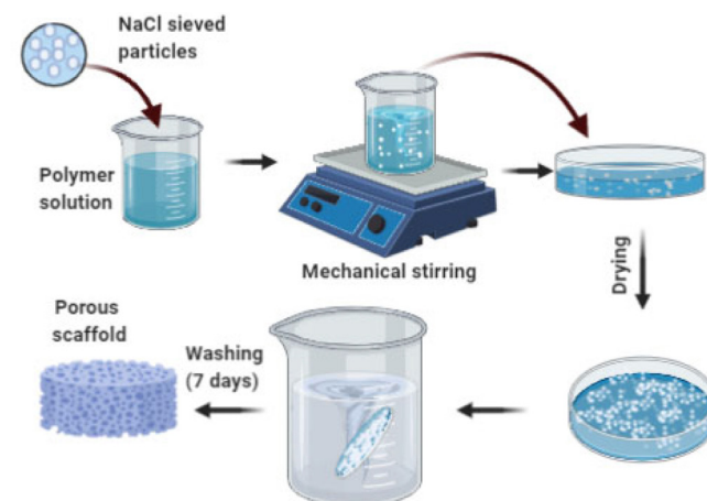
Figure 3. Illustration scheme of the leaching process
