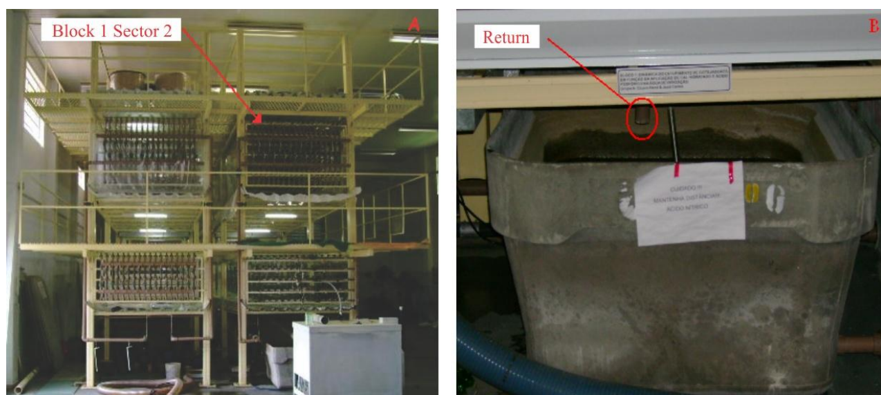
FIGURE 1. a) Detail of the sector where the experiment was run; b) Preparation tank of the solution [\text{Ca(OH)}_2] .
