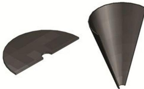
FIGURE 2. Flat bottom and conical hopper used.
