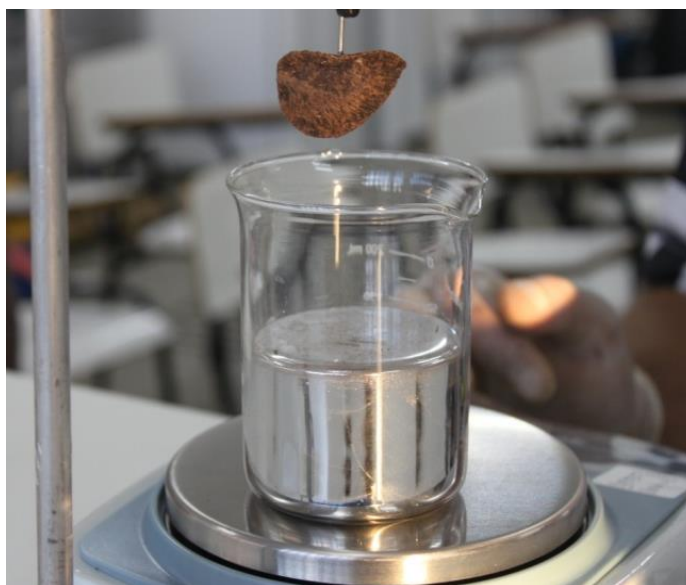
FIGURE 2. Determination of Unitary Specific Mass in the Brazil nut.
