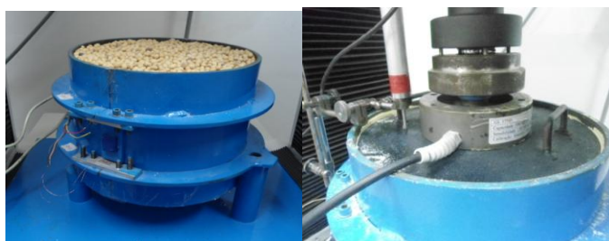
FIGURE 2. Cell instrumented and filled with grains.
