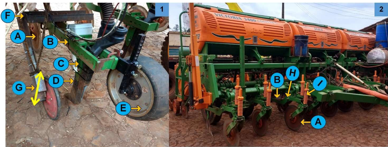
FIGURE 1. Detailing of the assembly set to measure furrowing shank strength and working depth. Legend: Cutting disc (A), fixing stringer (B), shank support (C), furrowing shank (D), limiting wheel (E), potentiometric sensor (F), and arm with wheel to contact the soil and measure shank depth (G). Coupling point (H) and compression spring (I).
