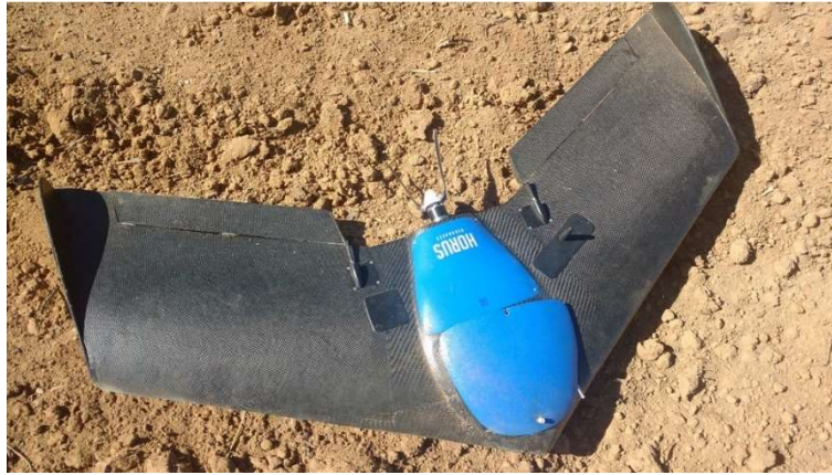
FIGURE 2. Remotely piloted aircraft (RPA) used for aerial survey, model ISIS, from Horus Aeronaves.
