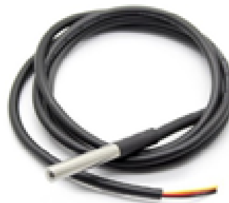
Figure 2. waterproof temperature sensor (DS18B20)
