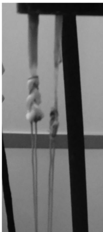
Fig. 10 - Region of suture failure in traction test
