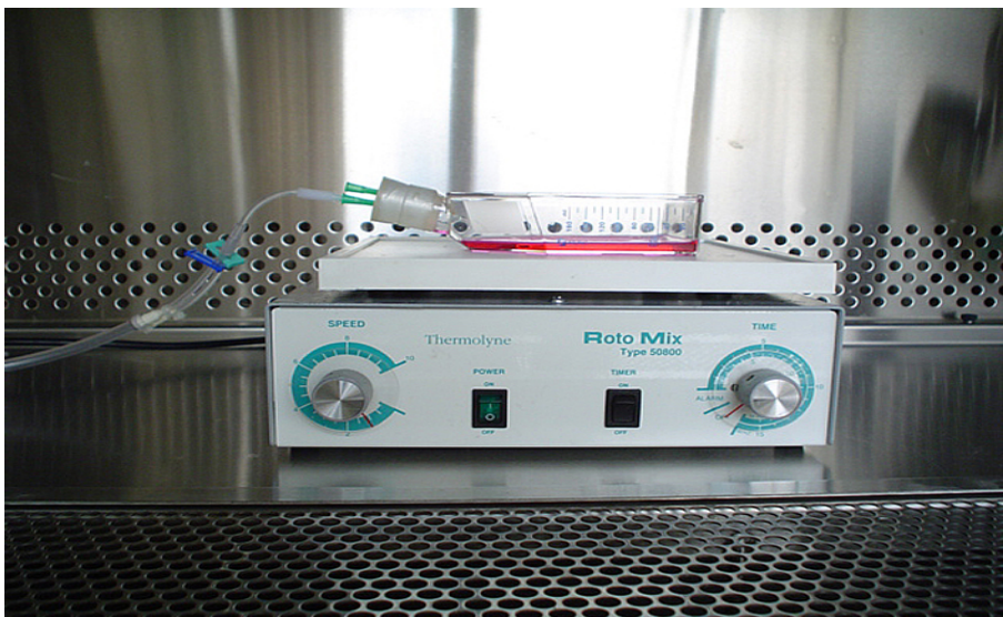
FIGURE 1 - Hypoxia system with gas mixture of 95% N 2 and 5% CO 2 consisting of gas torpedo, conductors of the gas mixture to the culture flask, inside a laminar flow system.
