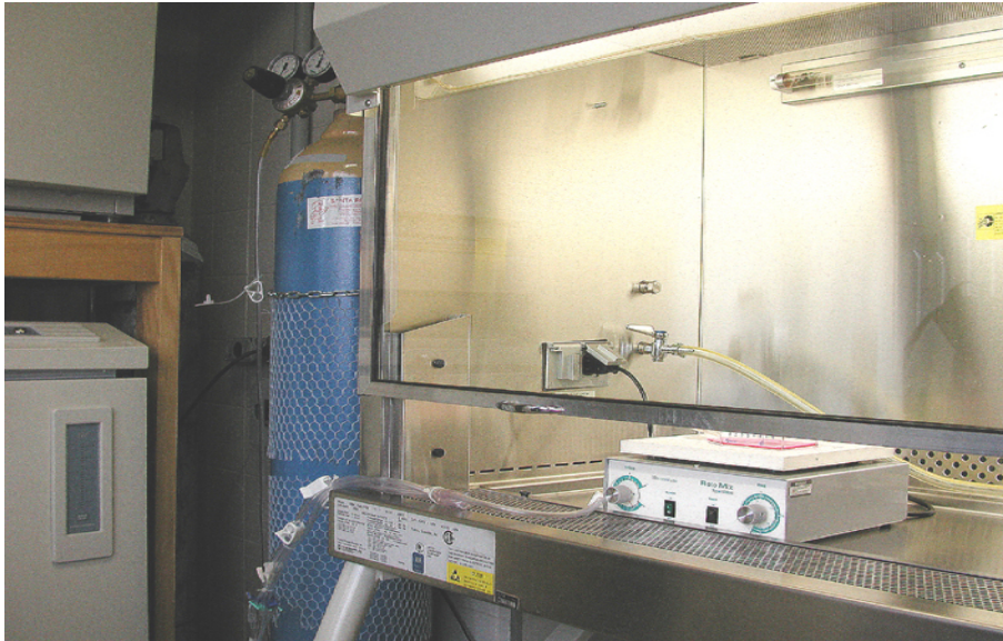
FIGURE 1 - Hypoxia system with gas mixture of 95% N 2 and 5% CO 2 consisting of gas torpedo, conductors of the gas mixture to the culture flask, inside a laminar flow system.
