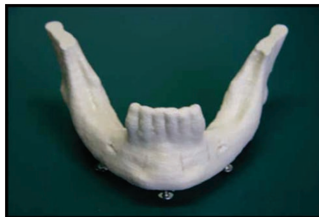
FIGURE 6 –Dentulous model produced by rapid prototyping
