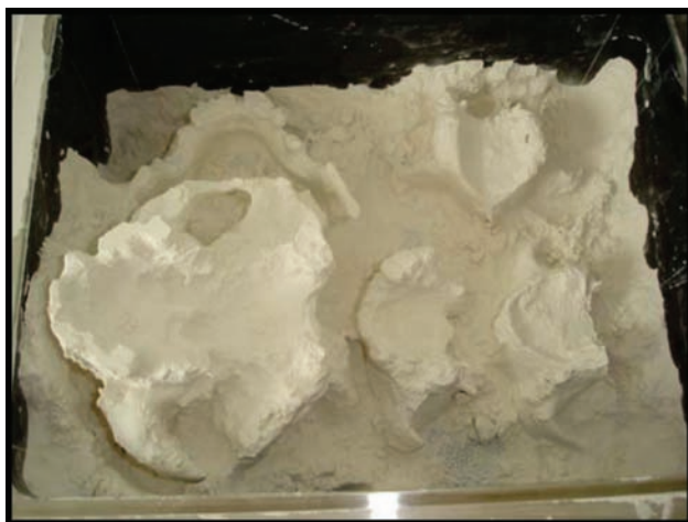
FIGURE 5 – Prototypes after the production, in the machine, without finishing
