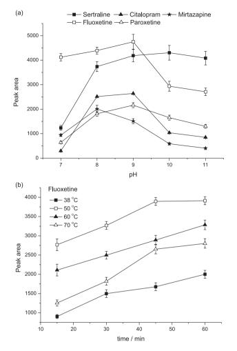
**Figure 1**. Optimization of the SBSE variables. (a) The effect of extraction pH on SBSE performance of all analytes, and (b) SBSE time extraction profiles for fluoxetine at different temperatures.
