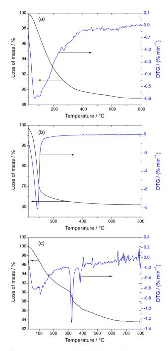
Figure 1. TGA profiles of (a) Na/Y; (b)Ni/Y and (c) [Ni(phen)<sub>2</sub>(H<sub>2</sub>O)<sub>2</sub>]/Y.
