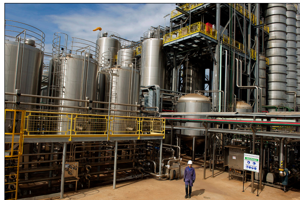
Figure 3. Amyris fermentation plant located in the city of Brotas, SP, Brazil. The 200,000 liter fermentation tanks are shown at the right of the picture.
