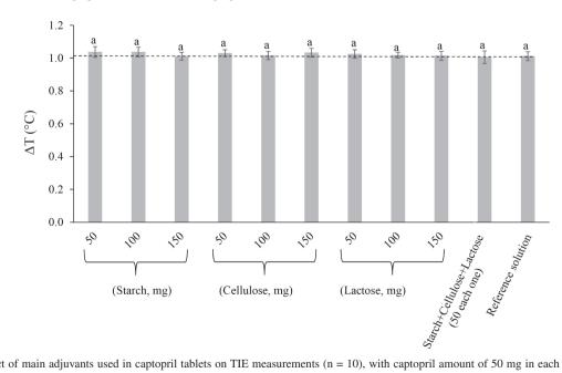
Figure 3. Effect of main adjuvants used in captopril tablets on TIE measurements (n = 10), with captopril amount of 50 mg in each well. Dashed line indicates the temperature of reference solution without adjuvants. Same letters indicate no significant difference (Tukey's test, p > 0.05).
