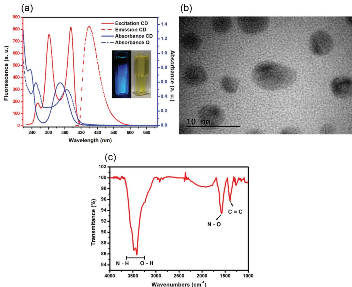
**Figure 1.** (a) An overlapping of absorption (—) excitation (---) and emission (---) spectra of the synthesized carbon dots and absorption spectrum of quercetin (---). The inset is the picture of carbon dots under light irradiation by a UV lamp at 380 nm (left) and without light irradiation (right); (b) A TEM image of the carbon dots synthesized; (c) FTIR (KBr) spectrum of CDs.
