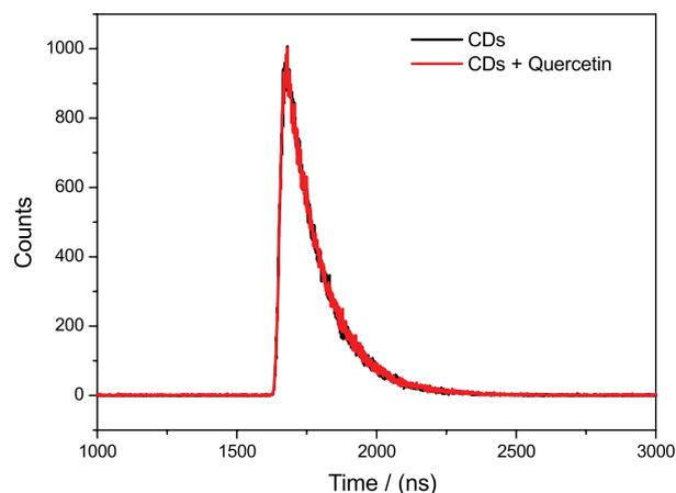
**Figure 7.** Fluorescence emission decay profile of the CDs and CDs in the presence of 10 mg L<sup>-1</sup> quercetin in buffer solution pH 11 ( $\lambda_{ex} = 380$  nm,  $\lambda_{em} = 450$  nm).
