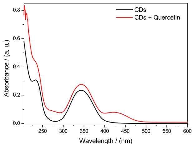
**Figure 6.** Absorbance spectrum of the CDs and of the product of the reaction between the CDs and quercetin.
