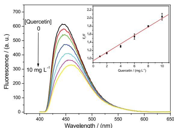
**Figure 4.** Fluorescence spectra for quercetin determination, reference solutions containing, 0; 1; 2; 4; 6; 8 and 10 mg L<sup>-1</sup>, the insert is the analytical curve for quercetin.
