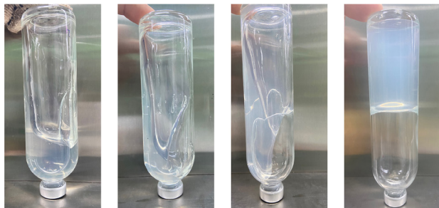
Figure 1. Illustration of the gelation progress of the gels. PPWG changing from strength A (left), to C, E, and H (right).
