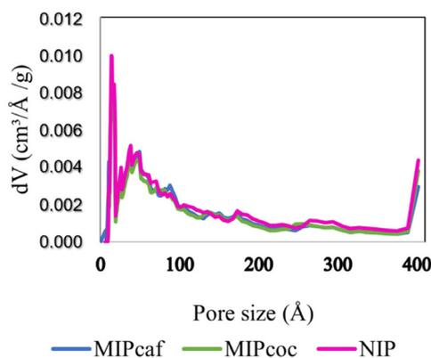
**Figure 3.** Pore size distribution of MIPcaf, MIPcoc, and NIP obtained by NLDFT.
