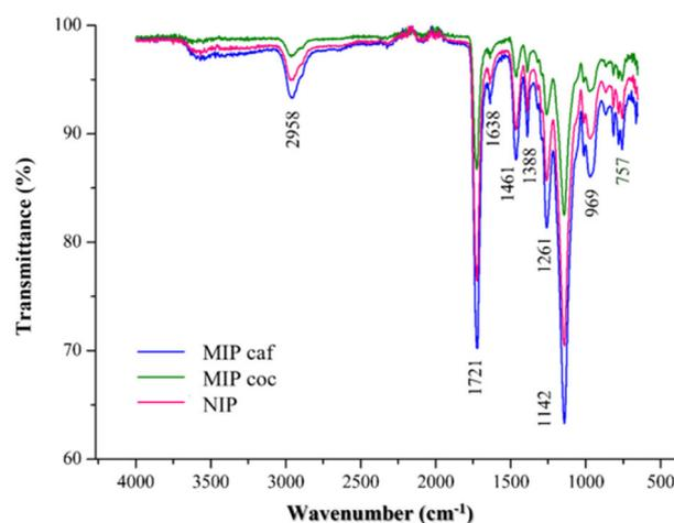
**Figure 4.** Infrared spectra (ATR) of the MIP synthesized from caffeine (MIPcaf), the MIP synthesized from cocaine (MIPcoc), and the non-imprinted polymer (NIP).
