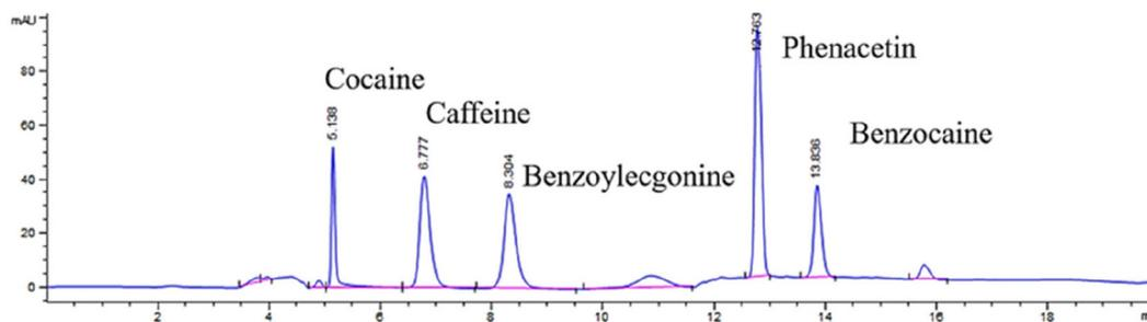
**Figure 5.** Chromatogram referring to the analysis of cocaine, caffeine, benzoylecgonine, phenacetin, and benzocaine using a  $C_{18}$  column (250 mm  $\times$  4.6 mm, 5  $\mu$ m), wavelength at 233 nm, mobile phase composed of ultrapure water (A) and acetonitrile (B), flow rate at 0.75 mL  $\text{min}^{-1}$  in gradient mode, as indicated in Table S8.
