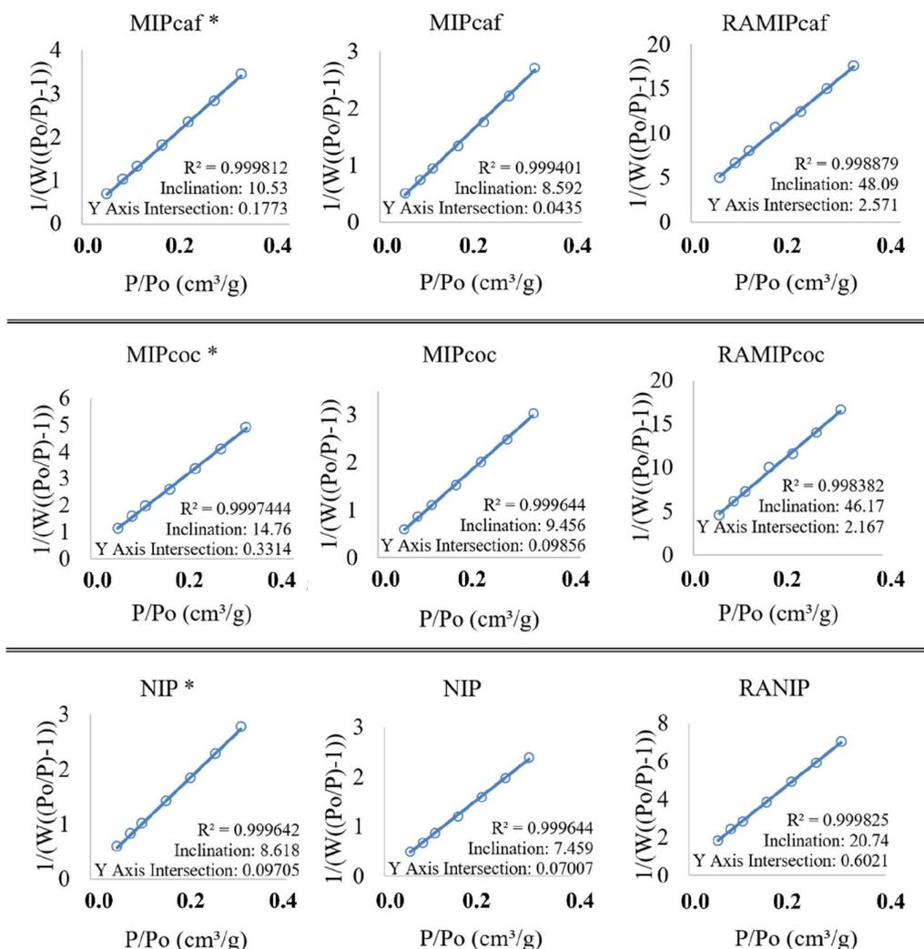
**Figure 2.** Analysis through the 7-point BET method of the adsorption curves for each polymer. \*Without washing.
