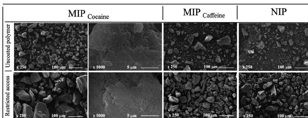
**Figure 1.** SEM images of the MIPs synthesized from cocaine and caffeine template molecules and NIPs. SEM images of the RAMIPs are also shown.
