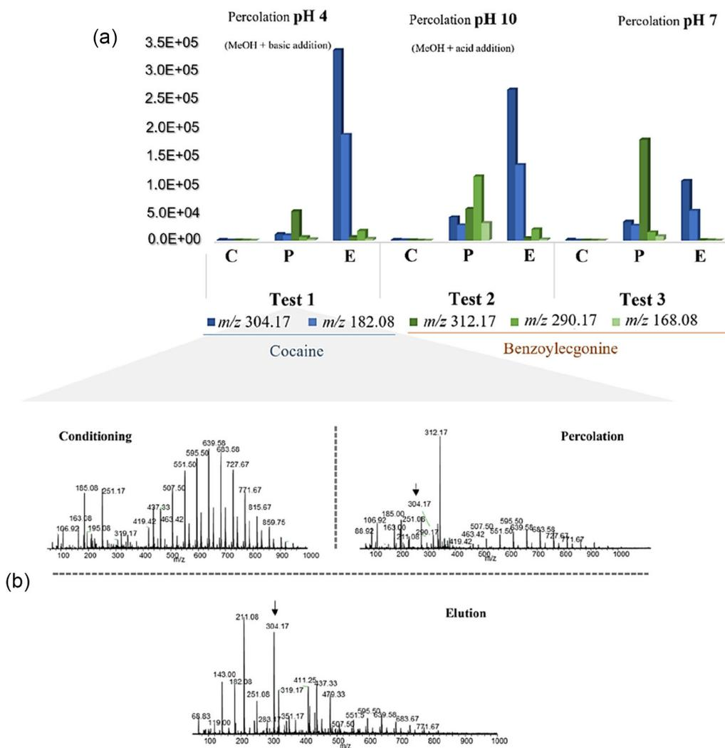
**Figure 6.** (a) Absolute intensity of signals related to the analytes in each extraction step: conditioning (C), percolation (P), and elution (E); (b) ESI(+)-LTQ-MS spectra of the conditioning, percolation using the sample at pH 4 and elution using methanol (with the addition of  $1 \text{ mol L}^{-1} \text{ NH}_4\text{OH}$  solution).
