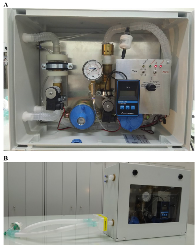
Figure 1 - Practical implementation of the ventilator. (A) Internal view showing the command panel and the main components. (B) External view with the attached standard double-limb respiratory circuit and, on top, the exhaust outlet and air and oxygen intakes (blue connectors).
