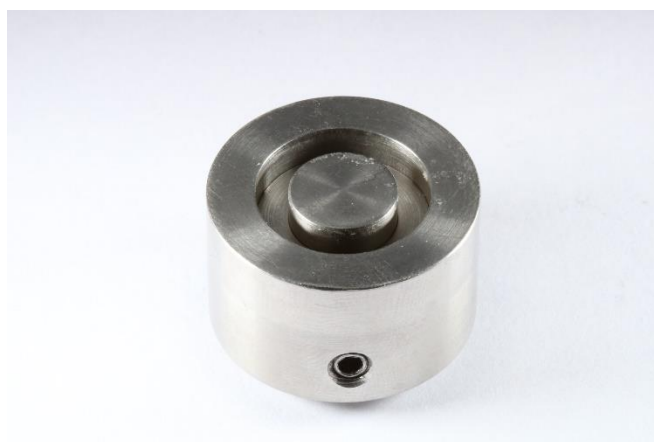
Figure 1. Metallic matrix used to build dual specimens.
