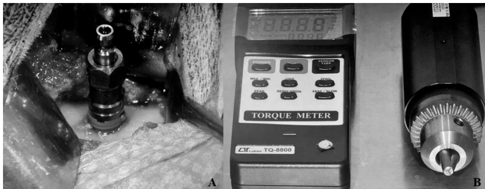
Figure 2. Representation of the biomechanical analysis that was assessed by the insertion and removal torque test. A) Implants placed in the native bone; B) The torque wrench used to apply the counterclockwise movement to remove the implants and obtain the removal torque forces
