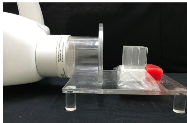
Figure 1. Representation of the standardization of radiographic acquisitions with the acrylic phantom and the image receptor.
