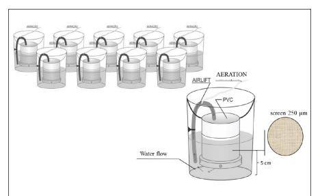
Figure 1 - Schematic of the experimental units used to evaluate the effect of stocking density on growth and survival of *Anomalocardia brasiliana* post-larvae.
