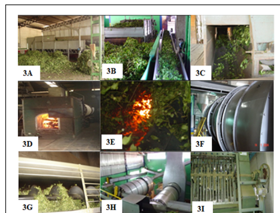
Figure 3 - Main stages of mate processing. 3A - Mate reception area; 3B and 3C - mate entering the process; 3D e 3E - mate sapeco ; 3F e 3G - mate drying; 3H - external view of the sapecador and mate dryer; 3I - mate crushing.
