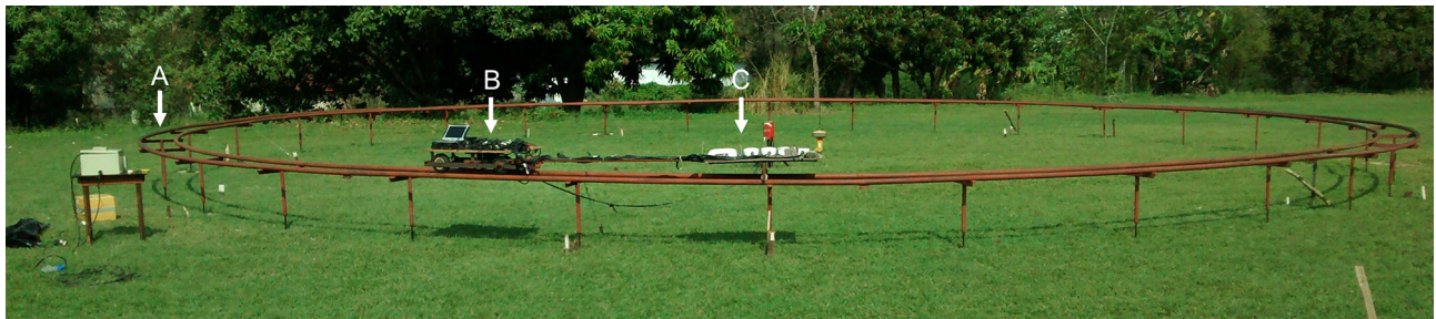
Figure 2 – Rail for the radial displacement of receivers (A); a platform with an electric motor (B) and platform for the allocation of GNSS receivers (C).
