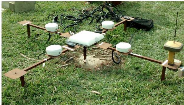
Figure 1 – Supporting frame to allocate GNSS receivers for the static test.
