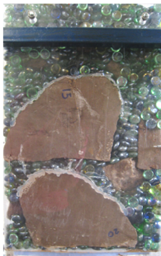
Figure 2: Column leaching experiment with large particles. Two large particles attached to the column walls are shown.
