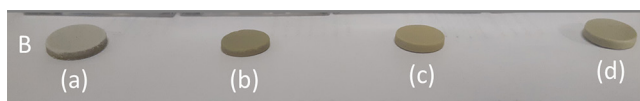
Figure 9: Images of glass B pellets before (a) and after thermal treatment for 1 h at: b) 892 °C; c) 1007 °C; and d) 1180 °C.
