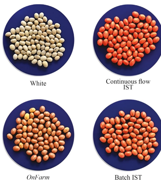
Figure 1: Visual appearance of the soybean seed treatments according to the application technology: continuous flow IST, batch IST, OnFarm and untreated control (white).
