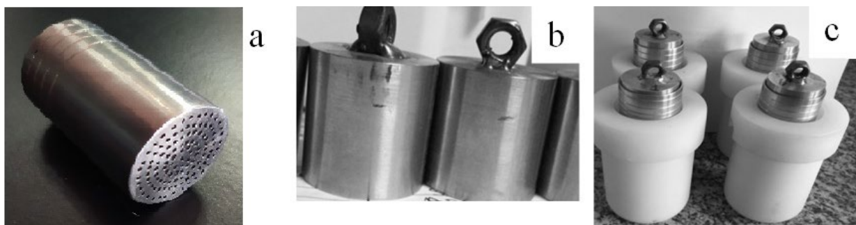
Figure 1: a: Stainless steel cylinders with draining bottoms; b: Stainless steel weights; b: Centrifuge tube holders with the cylinder, soil sample, and weights.
