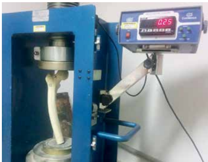
Figure 3. Manual hydraulic press used in the tests.
