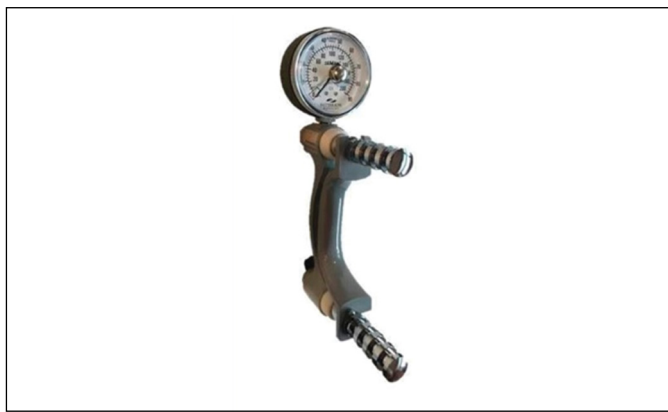
Figure 3. Manual pressure dynamometer used in the tests.
