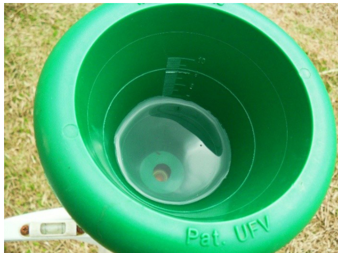
Figure 1. Water exposed to the atmosphere inside the evaporator
