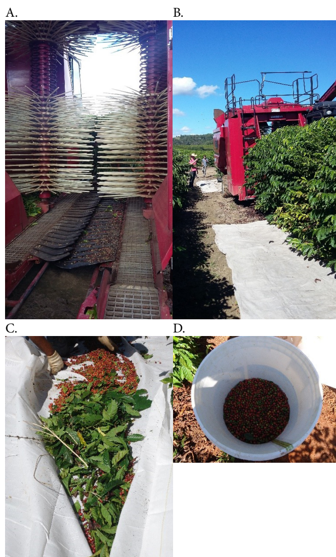
Figure 1. Self-propelled harvester used in the tests with detail of the unit of stripping and receiving the fruits (A), the cloths on the soil (B), the cleaning of fruits left on the cloths, but which would go to the ground (C), and measurement of fruit volume (D) in São Mateus, Brazil
