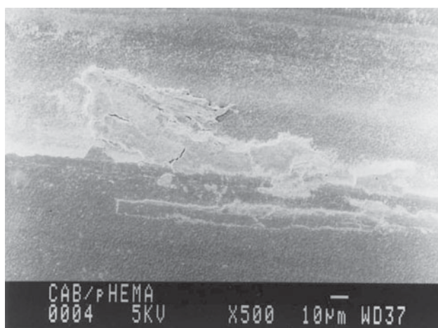
Figure 2. SEM worn surface of the pHEMA-CAB blend.
