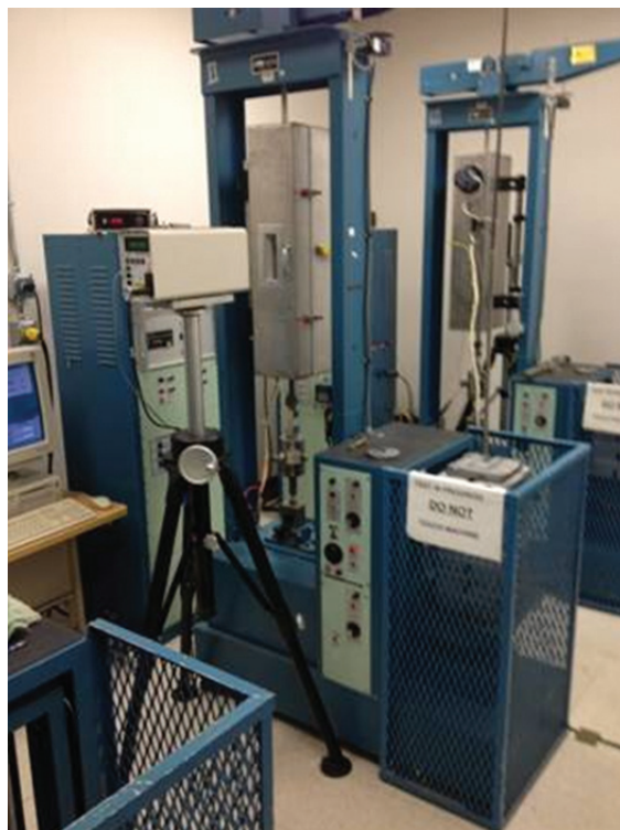
Figure 9. Creep machine and laser extensometer used for tests [Spirit Aerosystems].
