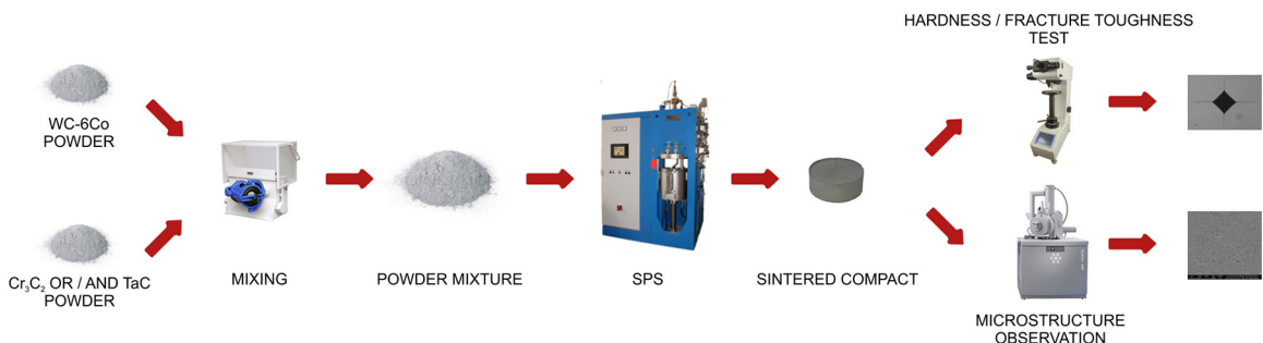
Figure 1. The scheme of the experimental procedure of the fabricating the WC-Co cemented carbide specimens and their examination.
