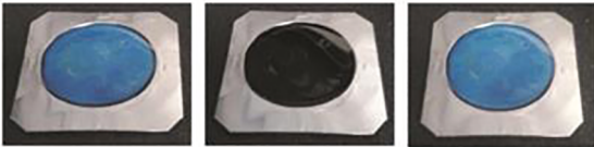
Figure 9. Color variation of LC in the temperature sensor prototype: on the left, heating from 80 to 90 °C; in the center, isotropic phase at temperatures above 100 °C; on the right, cooling from 90 to 80 °C.
