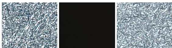
Figure 6. LC textures observed by PLM: (a) on heating; (b) isotropic and (c) on cooling.
