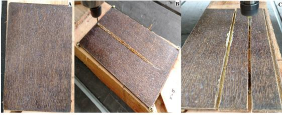
**Figure 5.** Jute/PP composite plate. (A) Jute/PP composite after processing. (B): Jute/PP composite plate cutting test on CNC machine. (C): Tensile testing specimen machining. Bibliographic source: Author.
