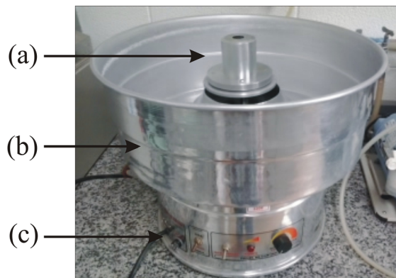
Figure 1. Image of the rotary jet spinning equipment used (a) central reservoir, (b) circular target, (c) base coupled to an electric motor
