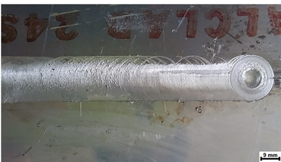
Figure 7. Variation in the final diameter of the weld bead of 18.37%, originated by the lack of rigidity of the vertical milling machine and high forging force variation at the end of the process.
