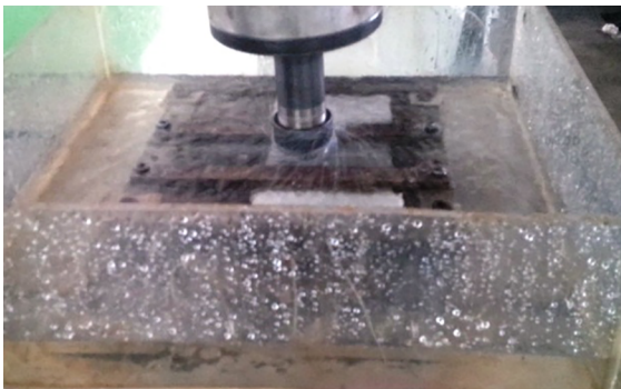
Figure 2 . Processing view of SFSW
